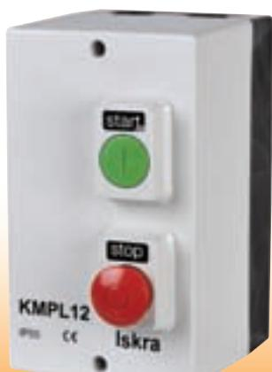
They are mainly used for start-up, overload protection and switch-off of electric motors and also for other loads. A contactor and a corresponding bimetal relay are built in the enclosure of degree of protection IP55. They are switched on with the ON pushbutton and switched off with the OFF pushbutton. The mushroom pushbutton functions as an emergency stop pushbutton.
